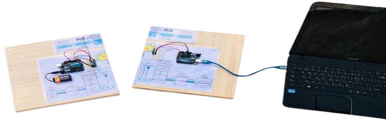
Fig. 9. The full system of transmitting and receiving digital information wirelessly at 433MHz
