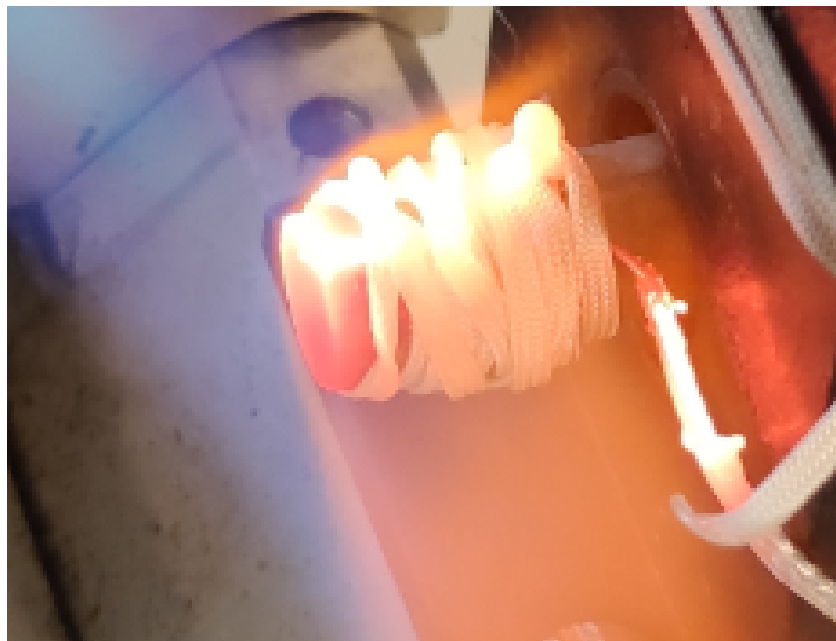
Figure 9. Probe and a thermocouple heated to 1100 °C.
