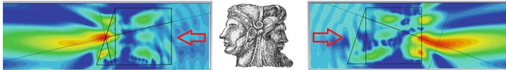
Fig. 2 The particle with broken symmetry for PH formation: the morphology of the field localization area depends on the orientation of the particle that resembles the two faces of “Janus bifrons”. Adapted from Ref. [33].
