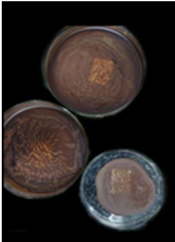
Fig. 2. Indicated SeNP particles-solution centrifuged at 8000rpm for 10 minutes
