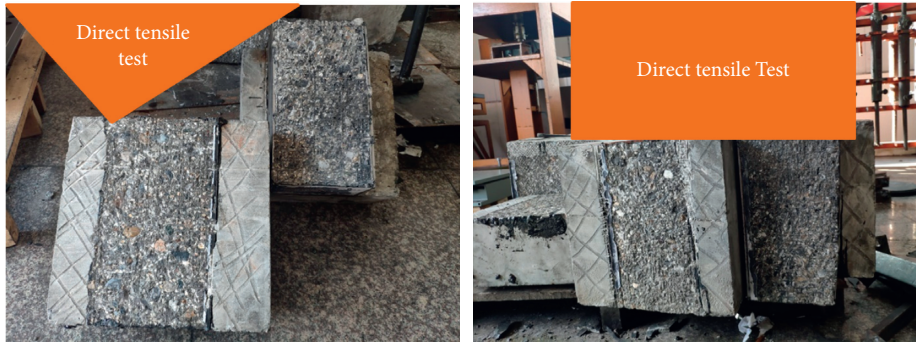
FIGURE 4: The failure mode of the direct tensile test specimen.
