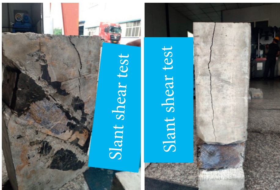
FIGURE 11: The failure mode of slant shear test specimen 3.
