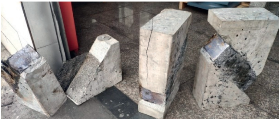
FIGURE 8: The failure mode of the slant shear test specimen.
