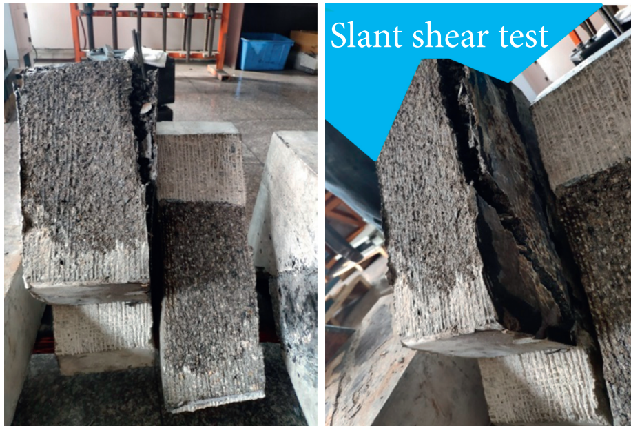
FIGURE 10: The failure mode of slant shear test specimen 2.
