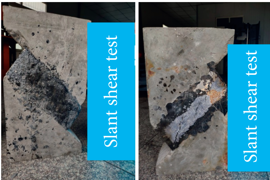
FIGURE 9: The failure mode of slant shear test specimen 1.
