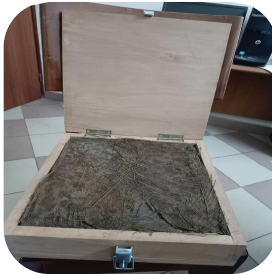
Fig. 7. Insulating panel sample with storage box
