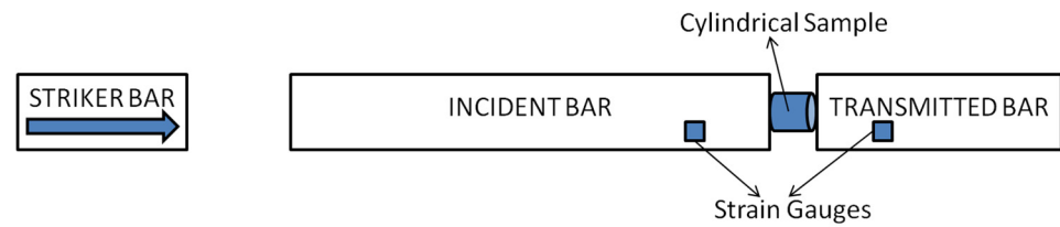
Figure 3. Schematic diagram of SHPB.
