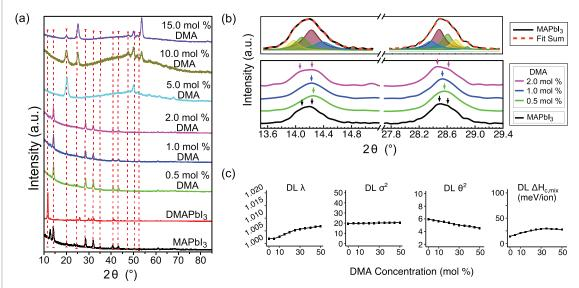
**Figure 8.** (a) XRD (x-ray diffraction) spectra of the synthesized  $MA_xDMA_1 _ xPbI_3$  thin films as a function of the DMA concentration. (b) High-resolution XRD spectra at selected peaks and the corresponding fit for MAPbI<sub>3</sub> (top panel) and for perovskites incorporating 0, 0.5, 1.0, and 2.0 mol% DMA (bottom panel). The arrows indicate the location of the main peaks. (c) DL predictions of the structural deformations in  $MA_xDMA_1 _ xPbI_3$ .
