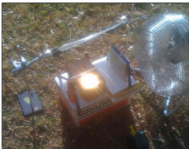
Fig. 9. Small-Area Fresnel solar concentrator apparatus with the brass target unpainted
