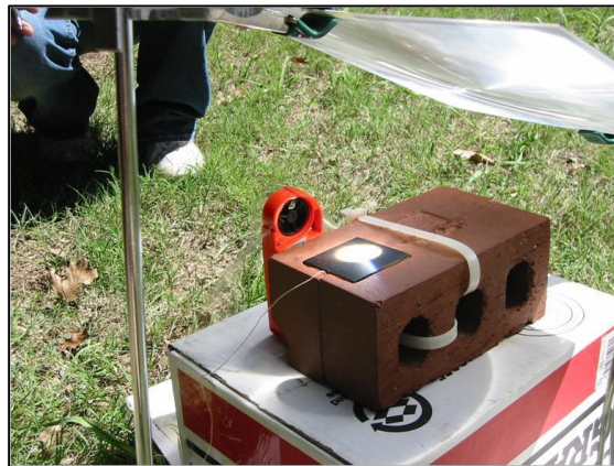
Fig. 10. Small-Area Fresnel solar concentrator apparatus with the brass target painted black.
