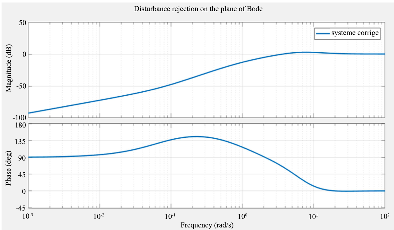
Figure 11. Response of the flow circuit on the plane of bode.
