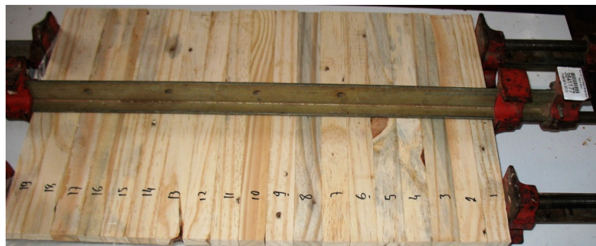
Fig. 2. Pressing procedure of the core battens
