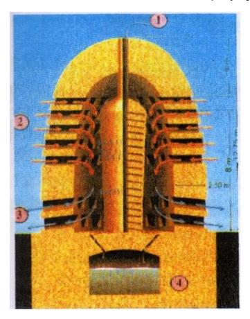
Fig. 2. Diagrammatic cut of the air well (1) top of the bell with the metal pipe which takes the air outside (2). Five lines of higher openings (3) Two lines of lower openings (4) Sat work and bulk storage tank of water. Document extracted the booklet of the Tourist office the Trans one in Provence
