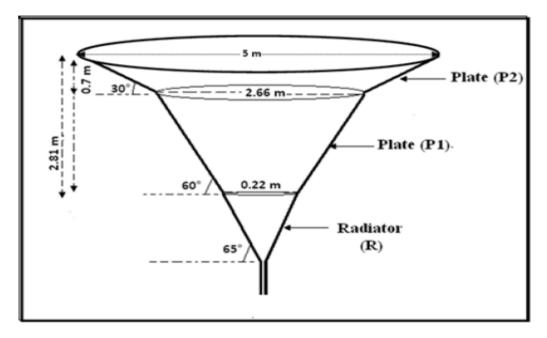
Fig. 7. The prototype of the experimental truncated cone condenser (Koto n'gobi, 2012)
