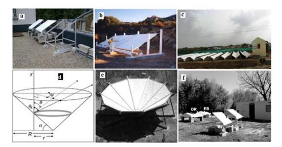
Fig. 5. (a) Installation of the planar condensers; (b) Vignola dew condenser; (c) Fully finished dew plant; (d) Integration scheme for the funnel shape (0<θ <θL, 0<φ <360 and 0 < r < R); (e) Photo of the funnel-shaped condenser (7.3 m surface area with 60 ° cone angle, 30 ° from horizontal); (f) "Egg Box" (EB) and "Origami" (OR) type condensers with the planar reference condenser (R). (T is an additional planar condenser)</li>
