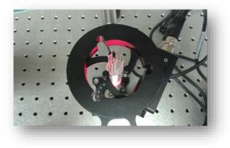
Fig. 3 Top view image of capillaries in a tube fixed in the FSP setup.
