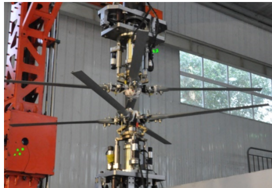
Figure 2. Installation of the upper and lower rotors in the test rig.
