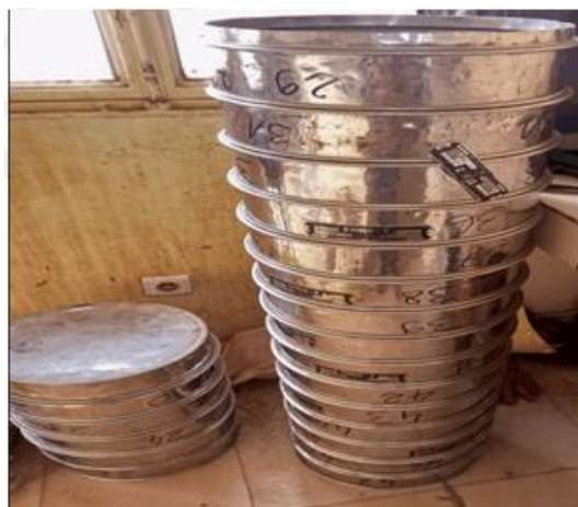
Fig. 1. Series of sieves for particle size analysis. Source: university of technology and management laboratory
