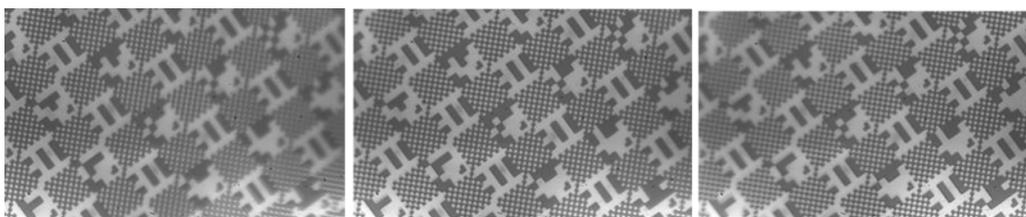
**Figure 9.** Observation of a portion of a nanoGPS tag with a 100× objective lens, with different focus settings: best focus at the left-hand side of the sample (left), in the center (center), at the right-hand side of the sample (right).
