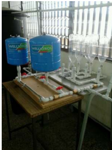
Fig. 2. Picture of pressure tank test assembly showing commercial pressure tanks and plastic bottle pressure tank of 10 L capacity
